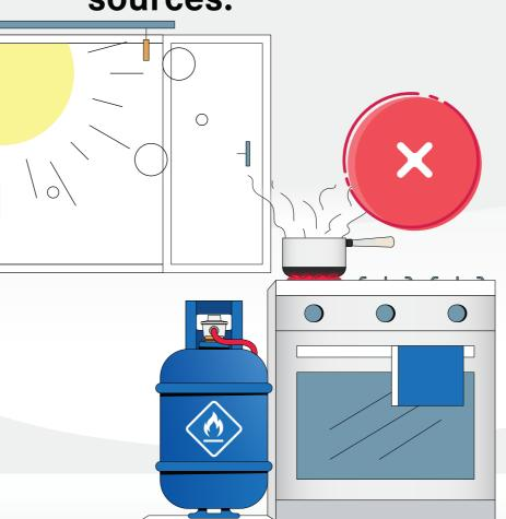
Do place the cylinder in a well-ventilated area.
